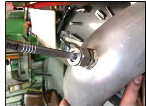
Coupon and UT sensor on an elbow
